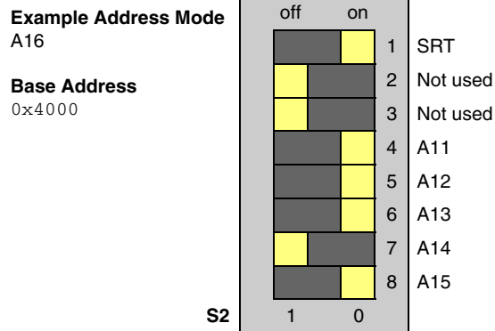
Figure 4. Setting the base address — Example (A16)
