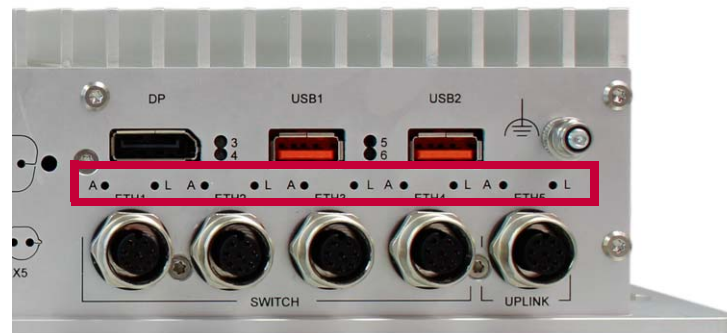
Figure 15. Position of Ethernet LEDs at BL50S front (highlighted in red)
