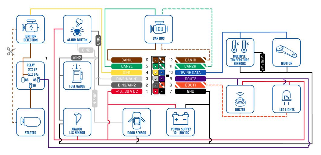
Figure 3 FMB140 Wiring scheme
