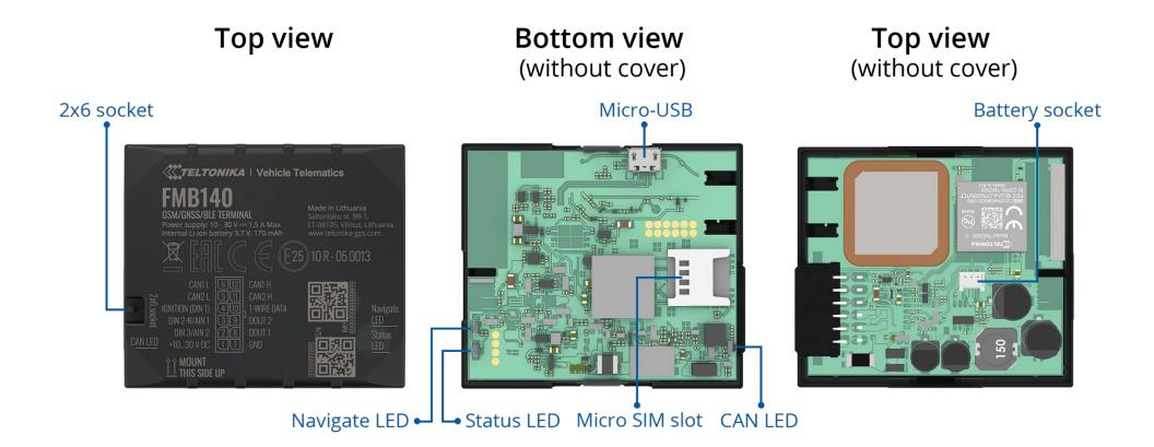
Figure 1 FMB140 device view
