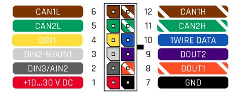
Figure 2 FMB140 2x6 socket pinout
