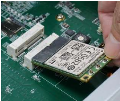
Insert on a 45 degree angle
