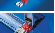
Keys are used for coding of board-type plug-in units and prevent the use of assemblies in incorrect slots. The keys are inserted into the chambers of the keyable guide rails and the injector/extractor handles, types IV, IVs and VII (4 positions are possible). This produces 64 keying combinations per guide rail
