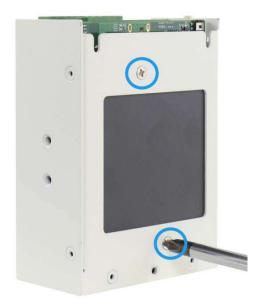
10. Install the cover, fasten the screws to secure the enclosure cover and cover plate.
