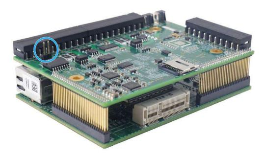
Jumper installed: resistance enabled
