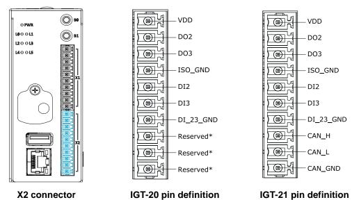
IGT-20/ IGT-21 Digital I/O Connector X2 Pin Definition
