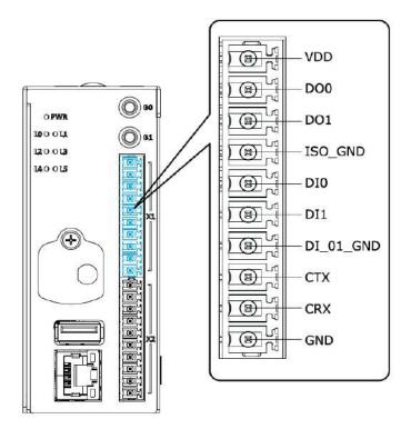
IGT-20/ IGT-21 Digital I/O Connector X1 Pin Definition
