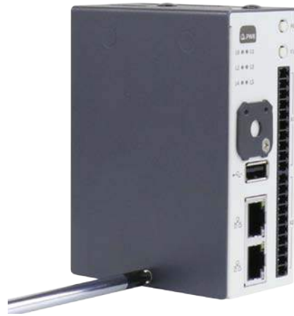
Fastening the cover screw
