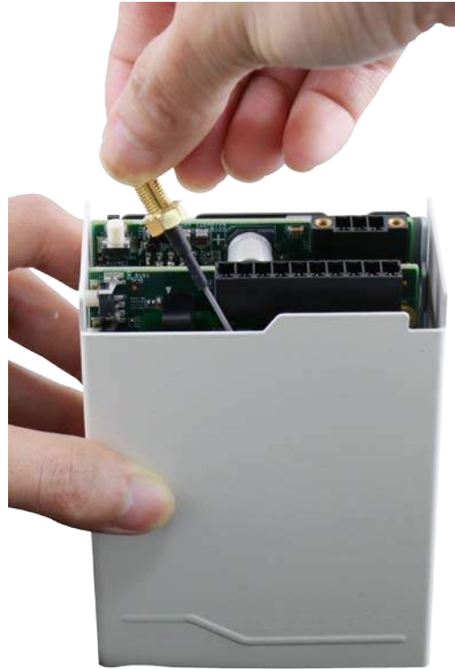
Make sure SMA female connector is accessible
