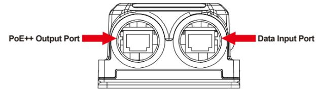
Figure 2-3: Two RJ45 Ports
