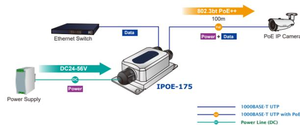
**Step 2:** The **PoE++ Out** port is the power injector which transmits DC voltage to the Cat5e/6 cable and transfer data from the Data source.
