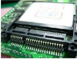
Installing the CFAST in the back of the board.
