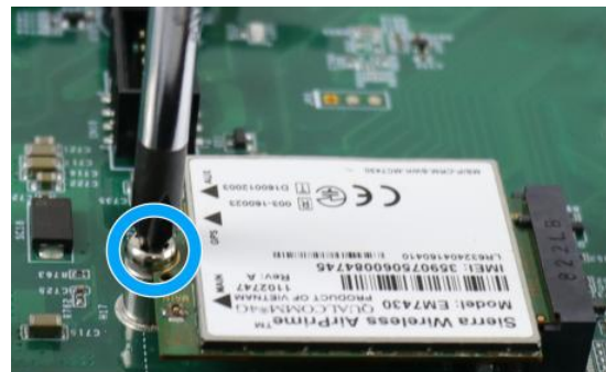
Secure with a M3 P-head screw
