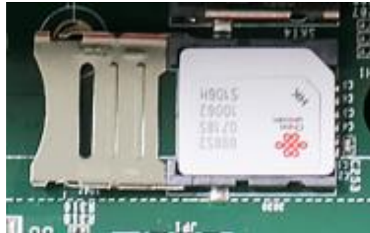
Flip-open the holder and place SIM
