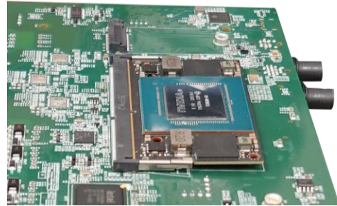
Press down to clip the module in place.
