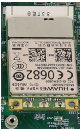
Insert at 45 degree angle
