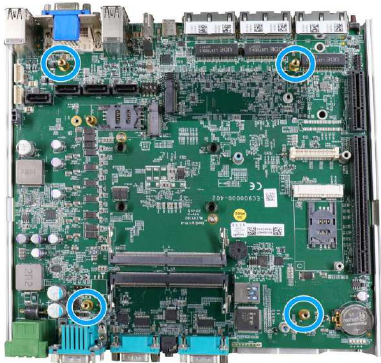
Secure motherboard with four screws
