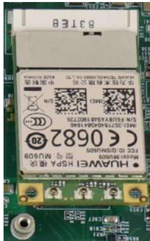
Insert on 45 degree angle
