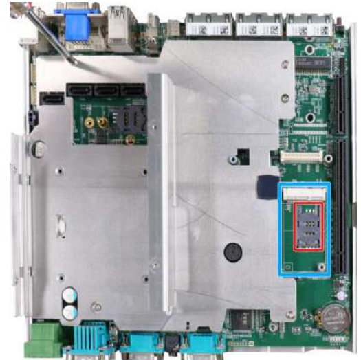
mini-PCIe slot on motherboard (underneath MezIO™ card)
