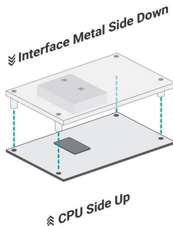
Rotate the module and heat spreader combo so that the I/O is facing the desired side, and place the combo in the position of the chassis reserved for your module.
