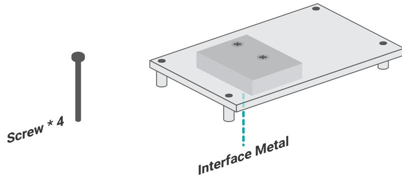
The heat spreader is designed to be mounted onto the module as illustrated below. Please make sure the contacting sides of the heat spreader and the module are correct – the CPU side of the module shall be facing the interface metal side and legs of the heat spreader. Rotate horizontally so the interface metal sits right on top of the CPU. Remove any plastic cover on the interface metal and apply thermal paste/adhesive if it is required.
