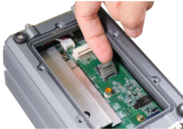
Slide to unlock the bracket Lift the bracket
