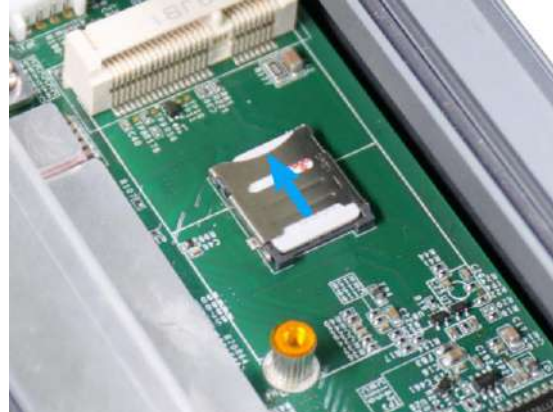
Slide to secure SIM and bracket
