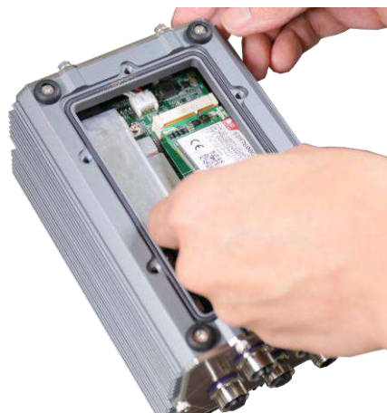
Insert at 45 degree angle
