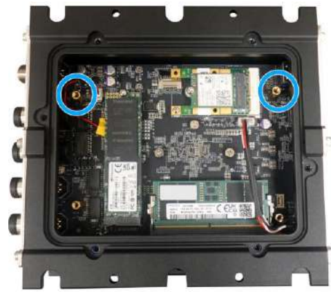
Install the copper stand-offs
