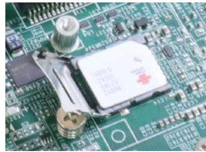
Flip open the holder and place SIM
