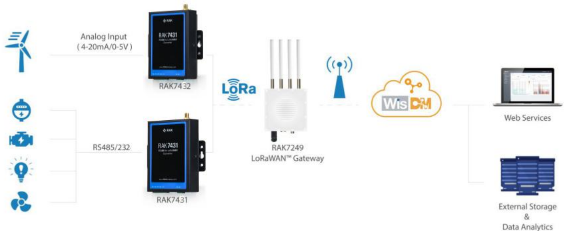
Figure 1 | RS485 to LoRaWAN™ network structure
