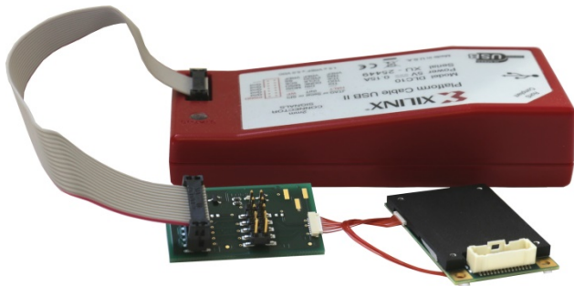
TMPE623 with TA308 & Platform Cable USB
