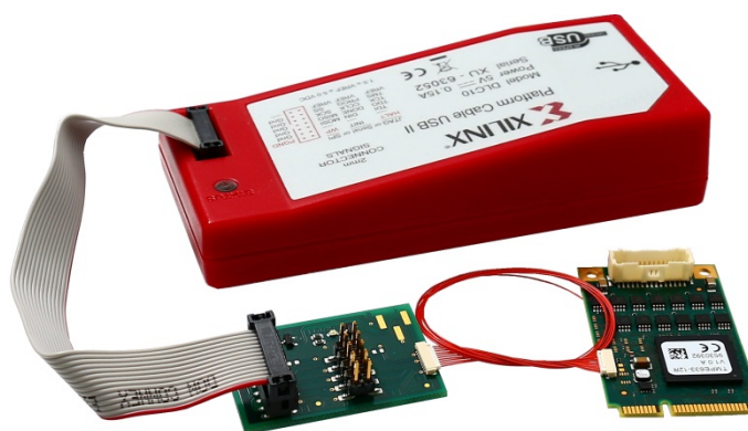
Figure 7-5: TMPE627 connected to a Programmer via TA308
