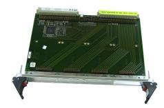
The M-Modules are screwed tightly on the carrier board, but the board needs only one slot on the VMEbus. Please note that since all three rows of the P2 connector are used for user I/O, board models with this connector are not compatible with VME64 backplanes. An interrupt controller handles the M-Modules individually. In VMEbus D16 systems the I/O signals of the M-Modules can be accessed from P2/J2 inside the rack.
