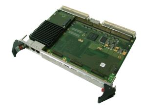
Its sister card, the A21C, offers two PMC/XMC slots instead of M-Modules, for different I/O requirements. Where there's a need for even more or other I/O, the A21B also includes a custom I/O mezzanine card option that reduces the board by one M-Module but provides interfaces like USB 2.0, COM or even custom I/O controlled by the onboard FPGA. The mezzanine card is always an entirely customized adapter PCB, including front I/O, and makes the A21B a semi-custom solution.
