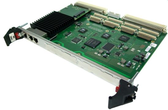
The A21C is an NXP (formerly Freescale) QorIQ based single-board computer for embedded industrial applications. The SBC features full VME64 support and can be used as a master or a slave in a VMEbus environment. The A21C provides 1 MB local dual-ported SRAM for slave access and communication between the local CPU and another VMEbus master.
