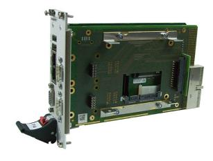
The F600 is a 4HP legacy I/O extension card for 3U Intel<sup>®</sup> based CompactPCI<sup>®</sup> single-board computers. It can be used in combination with the F14 and compatible CPU boards.
