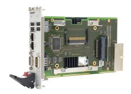
The F603 is a 4HP mixed USB/COM extension card for 3U Intel® based CompactPCI® single-board computers. It can be used in combination with the F14 and compatible CPU boards.
