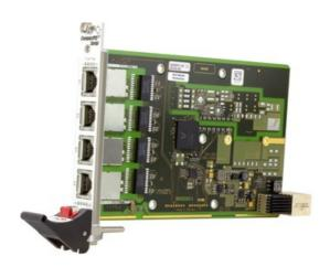
The GP1 is a 3U Gigabit Ethernet PHY line card, with optional PoE support, implemented as a CompactPCI® Serial board. It occupies one peripheral slot using a 4 HP front panel with four Gigabit Ethernet ports on RJ45 connectors. Alternatively, the GP1 can be supplied with four M12 connectors on the front panel (X-coded variants in preparation).
