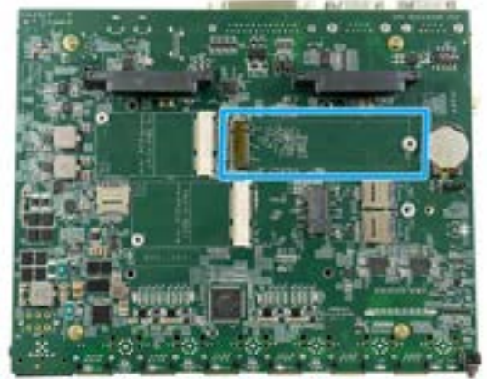
Location of M.2 M key socket (heat spreader removed)
