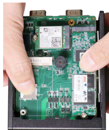
Secure micro SIM with cover
