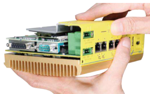
Install I/O panel
