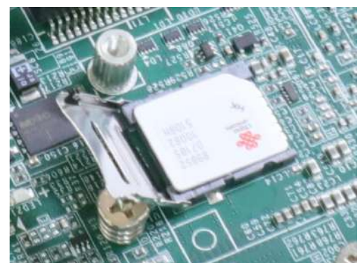
Push the SIM holder in the direction shown Flip open the holder and place SIM
