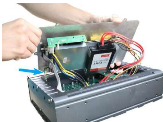
Disconnect the 4-pin power connector
