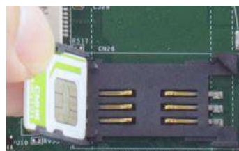
Insert SIM card with pins facing up
