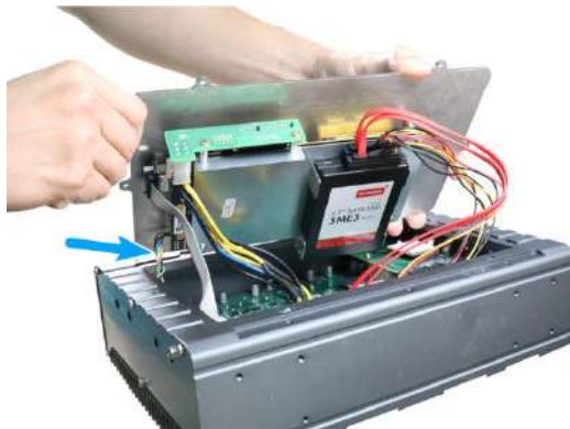
Connect the 4-pin power connector
