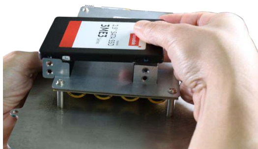
Place hard drive in between brackets
