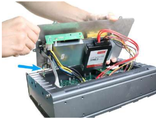
Connect the 4-pin power connector
