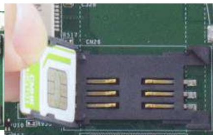
Insert SIM card with pins facing up
