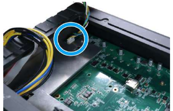
Unplug the 4-pin ATX connector
