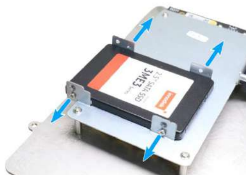
Remove screws on both sides of the hard drive
