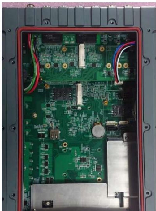
O-ring seated properly in the groove
