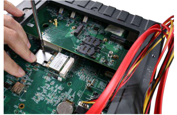
Secure the module with a screw
