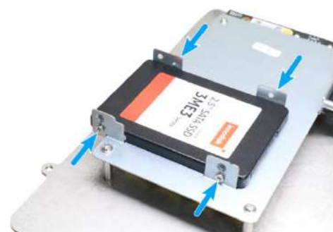
Secure hard drive with screws on both sides
