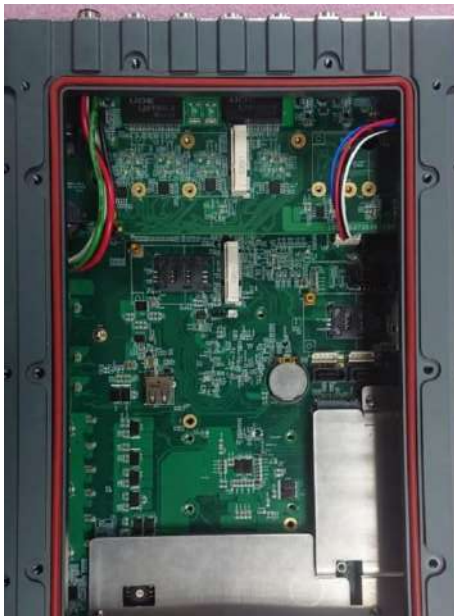
O-ring seated properly in the groove
