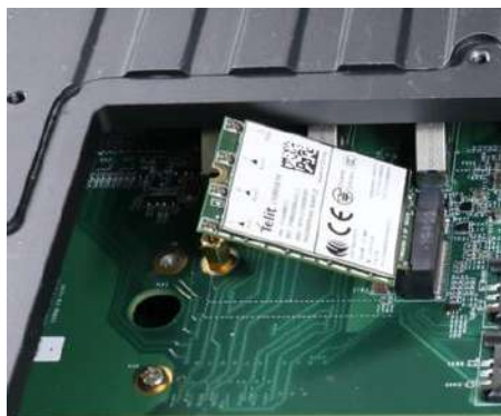
Insert into slot on a 45 degree angle
