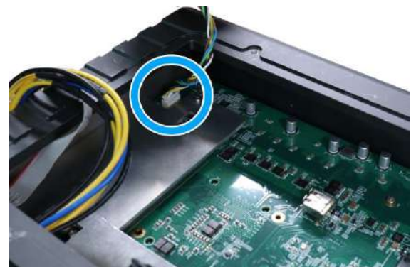
Unplug the 4-pin ATX connector
