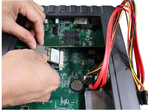
Insert into slot on a 45 degree angle
