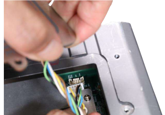
Connect from the motherboard side
