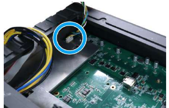
Unplug the 4-pin ATX connector
