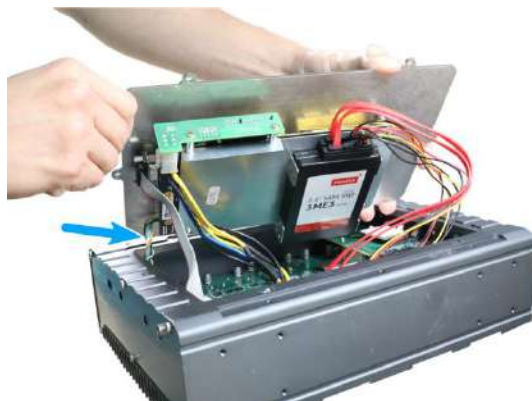
Disconnect the 4-pin power connector
