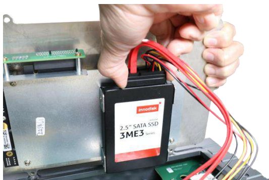
Disconnect the SATA/ power connector
