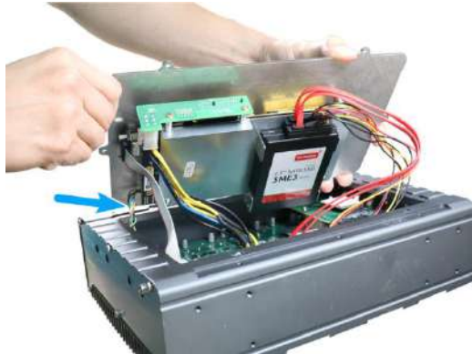
Connect the 4-pin power connector
