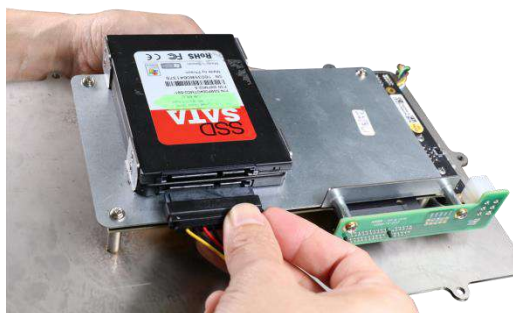
Connect the bottom hard drive first
