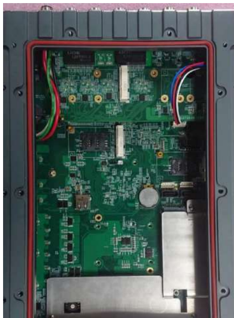
O-ring seated properly in the groove
