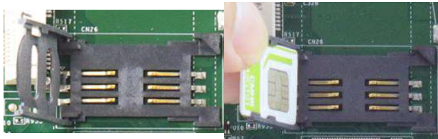
Slide and lift SIM card holder
