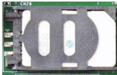
Secure the SIM card by sliding the holder
