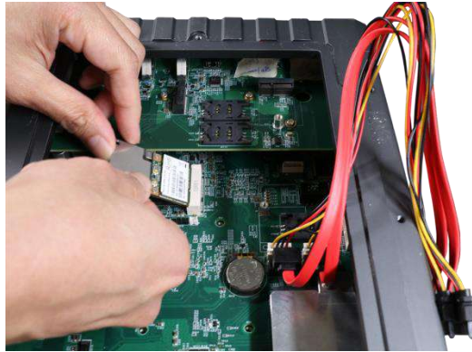
Insert into slot on a 45 degree angle
