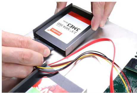
Disconnect the SATA/ power connector
