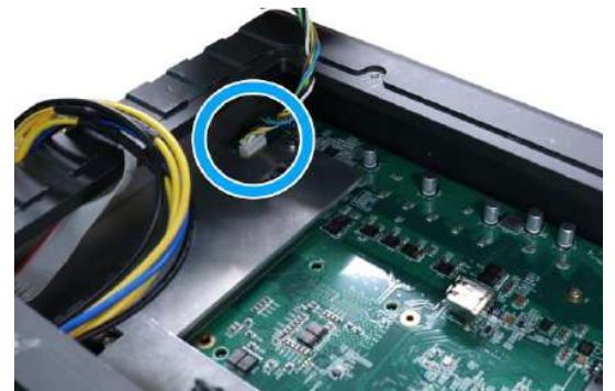
Unplug the 4-pin ATX connector
