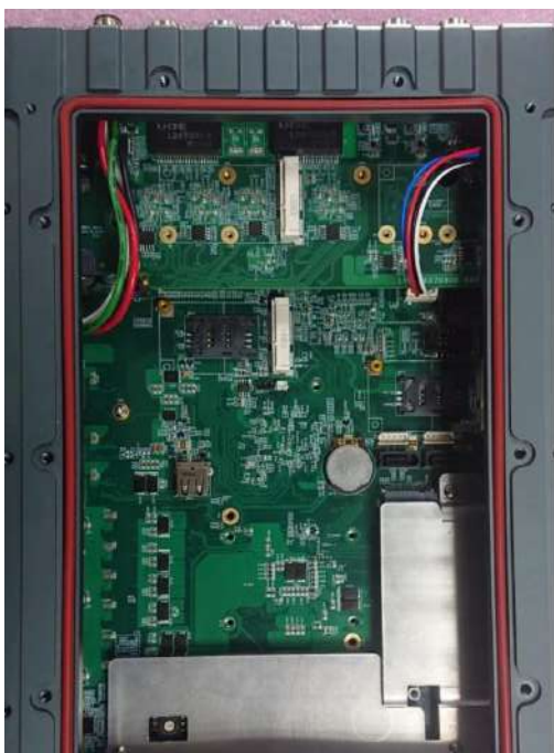
O-ring seated properly in the groove
