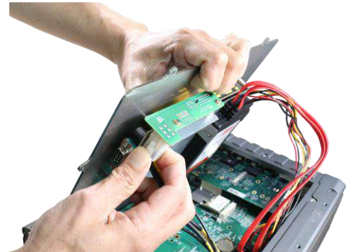
Unplug the 4-pin ATX connector
