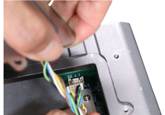
Connect from the motherboard side
