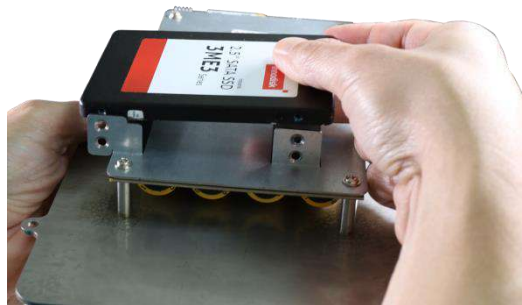
Place hard drive in between brackets
