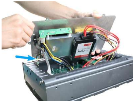
Connect the 4-pin power connector
