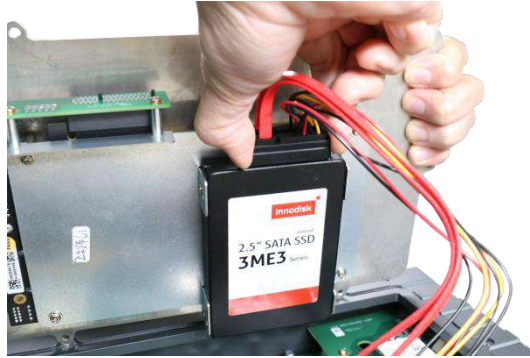
Disconnect the SATA/ power connector
