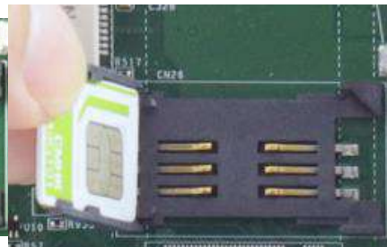
Insert SIM card with pins facing up
