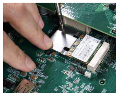
Secure the module with a screw
