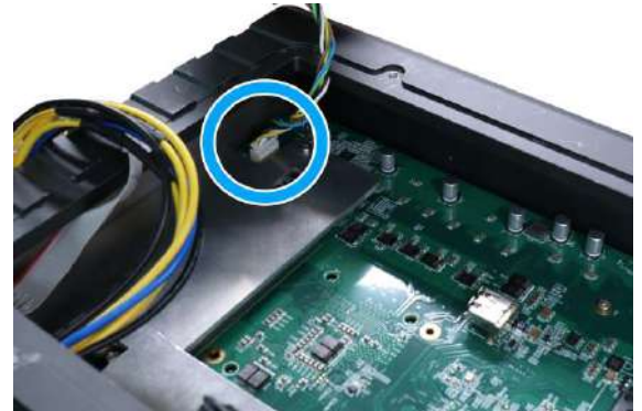
Unplug the 4-pin ATX connector
