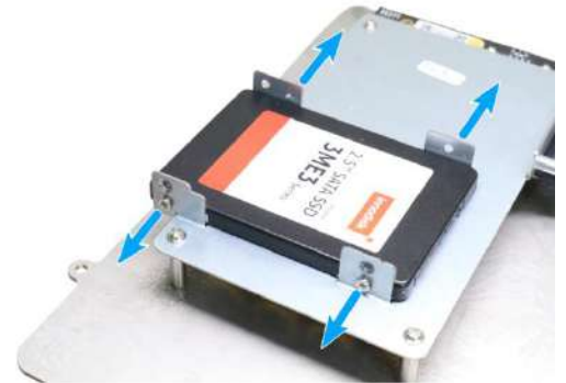
Remove screws on both sides of the hard drive
