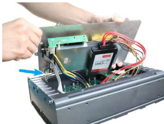
Disconnect the 4-pin power connector
