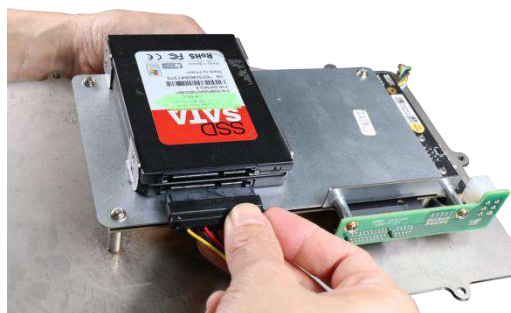
Connect the bottom hard drive first
