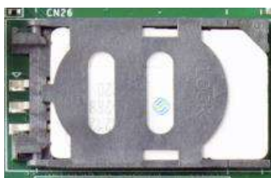
Secure the SIM card by sliding the holder
