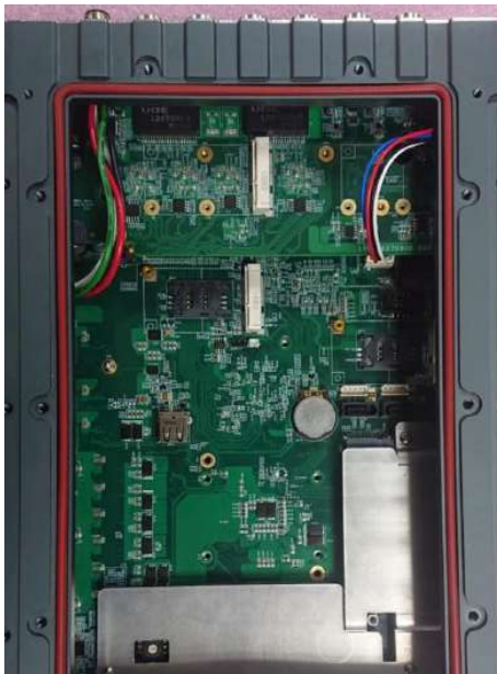
O-ring seated properly in the groove
