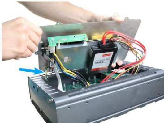
Disconnect the 4-pin power connector
