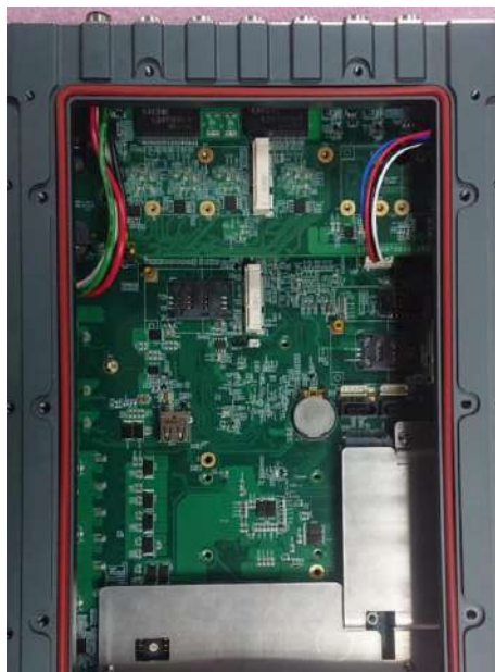
O-ring seated properly in the groove
