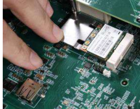
Secure the module with a screw
