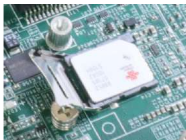
Flip-open the holder and place SIM
