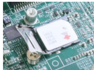
Flip-open the holder and place SIM
