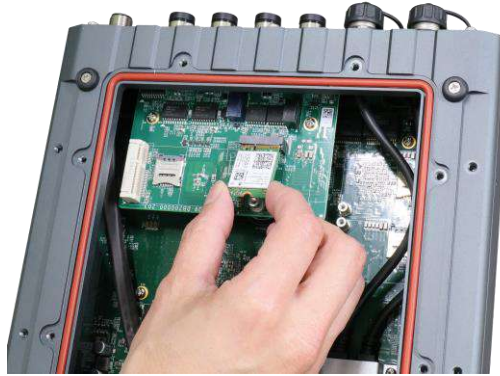
Insert on a 45 degree angle
