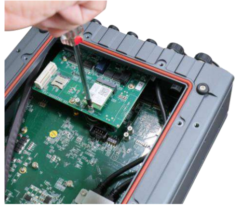
Secure with a screw
