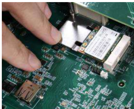
Insert into slot on a 45 degree angle Secure the module with a screw
