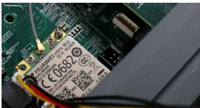
Insert into slot on a 45 degree angle Secure the module with a screw
